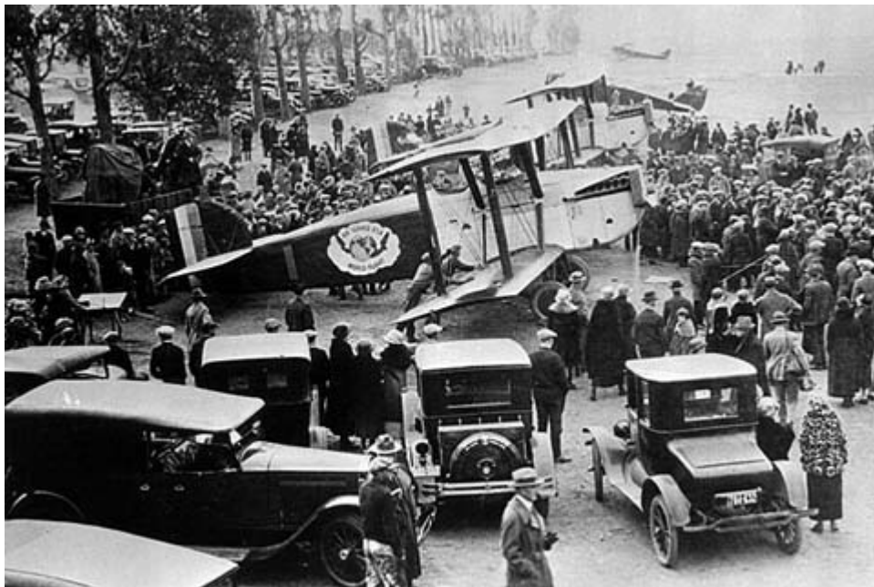
Built in 1924, the Douglas World Cruiser was a two-place biplane with a 50-foot wing span, powered by a 420 horsepower Liberty engine. (Photo Courtesy of Boeing)
